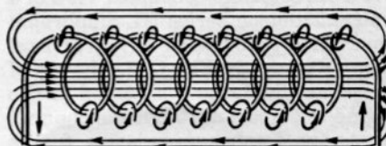
Fig. CS12—When a wire carrying an electrical current is wound in the shape of a coil or helix, the magnetic field surrounding loops of the wire tend to converge into a single electro-magnetic field as shown. If the loops of the coil are wound closely together, there is very little tendency for the electro-magnetic field to surround individual loops of the coil.
