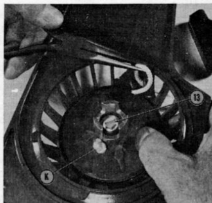
Fig. HL121—Pulling loop of starter rope past notch in rope pulley. Rope is retained by knot (K). Rope pulley retaining screw is (13).
